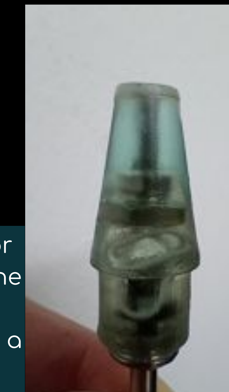
Figure 4. Sensor tip (frontal view). Central electrode configuration used for localized impedance measurements.
