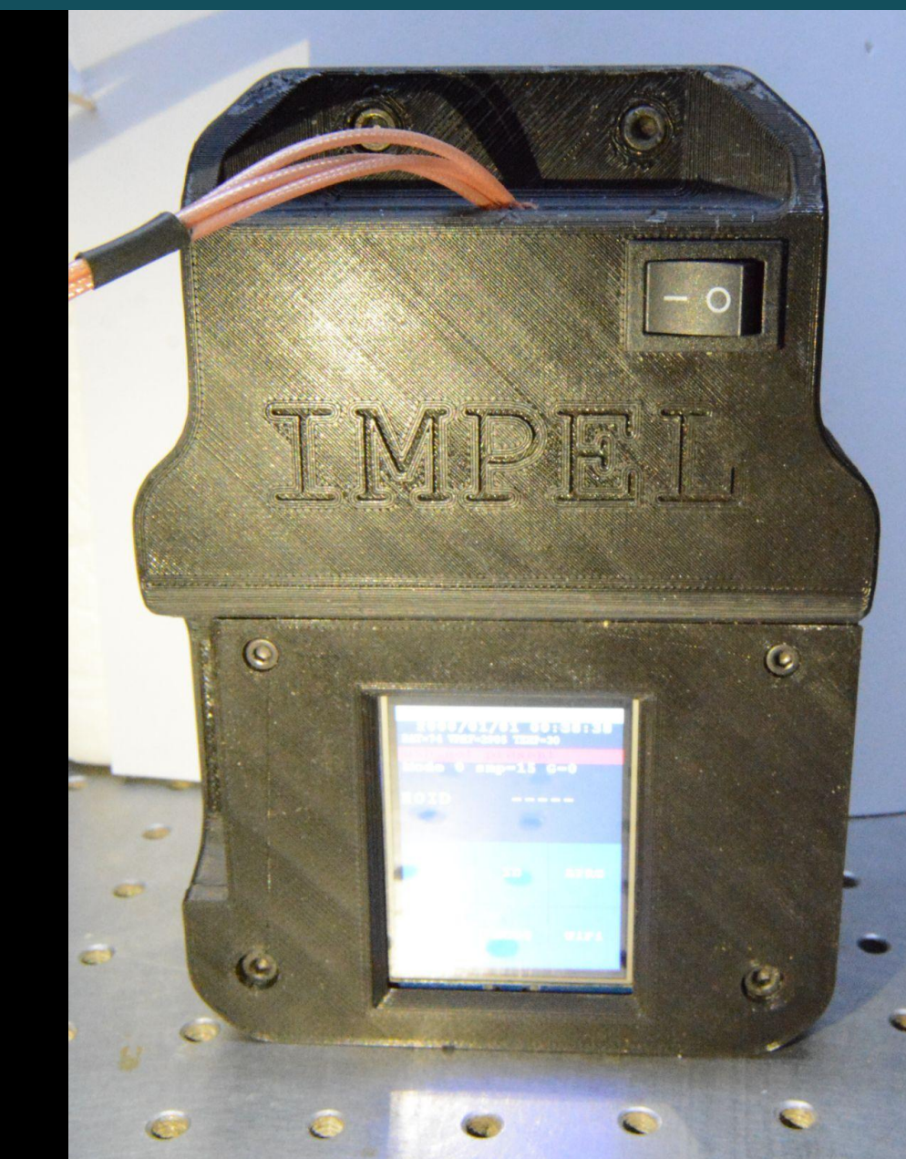
Figure 2. Ocular surface sensor. Sensor designed for controlled contact with the ocular surface, enabling stable acquisition of electrical signals across a wide frequency range.
